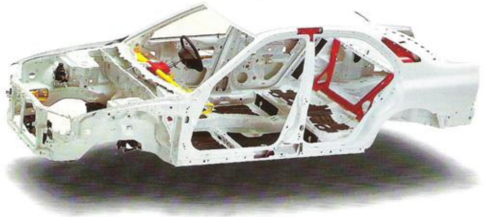
Rigid unit-body construction enhances safety and handling while also dampening noise and vibration
