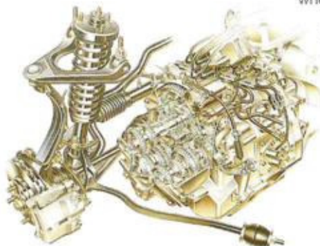
Front double wishbone suspension and automatic transmission
