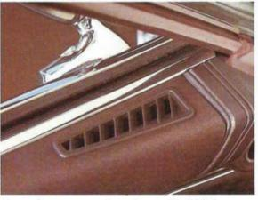
An air duct extension from the windshield defroster directs a stream of air against both door windows to help keep the glass clear in cold or muggy weather.
