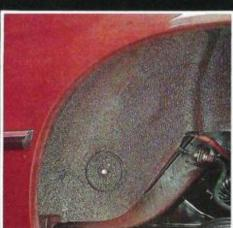
Special undercoating material helps protect the Accord's body from dust or moisture, also helps deaden road noise and retards rust.
