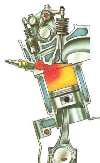
The Accord's CVCC Advanced Stratified Charge Engine is remarkably efficient. It needs no air pump, exhaust gas recirculation system, or expensive catalytic converter.
