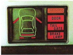
This lighted diagram lets you know at a glance if the doors or rear hatch are not securely latched. It also warns you if either stoplight should fail.
