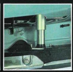
The bumpers, both front and rear, on the Accord are designed with rugged, built-in hydraulic shock absorbers to minimize sheet metal damage in minor traffic mishaps.
