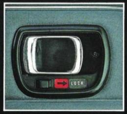
The inside door locks on the Accord have color-coded tabs...lets you check at a glance to be sure doors are locked.
