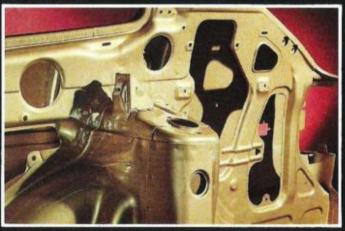
Unitized body construction helps make the Accord a very solid car, yet saves hundreds of pounds of unnecessary weight.
