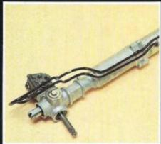
The Accord's rack and pinion steering provide light, positive steering control with a minimum of driver effort. Variable assist power steering is provided as standard equipment on the Accord LX.
