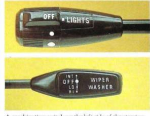
A combination switch on the left side of the steering column controls headlights and directional signals. The lever on the right operates the wipers and windshield washers.
