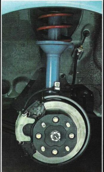
Both front and rear suspension on the Accord incorporate MacPherson struts. Long, resilient coil springs with integral double-acting shock absorbers smooth out the bumps. Power-assist front disc brakes help provide smooth stops.
