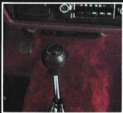
The standard transmission in both the Accord or the Accord LX is a 5-speed unit, with synchromesh in all forward speeds. Fifth gear is actually overdrive, which reduces engine speed at highway cruising.
