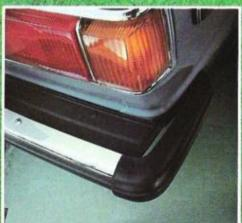
The energy-absorbing bumpers on the Accord have been redesigned for 1978. Notice the added protection provided by the new bumper end extensions.
